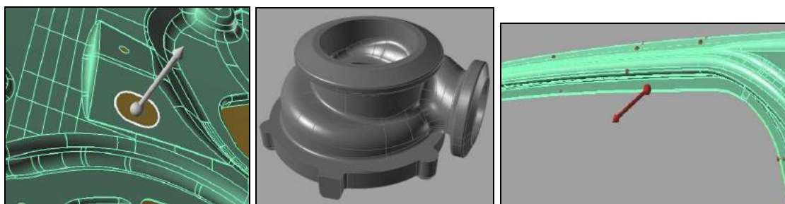
Fig. 2: Examples of inspection tasks: sheet metal cutout border acquisition (left, task of type b), global shape inspection (in the middle, task of type d), and specific target point assessment marked with red dot and arrow (on the right, task of type e).
