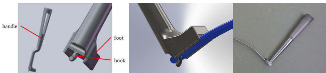
Fig. 3: Final design: whole tool, hook and lever arm (left), simulation of the tool-bar engagement (middle), metal prototype engaged with the pectus bar (right).
