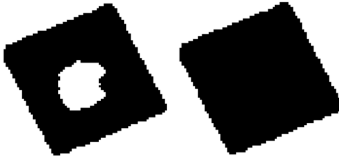
Fig. 4: Sample metric computation for connected component x,y with fiducial present. The black/white regions have been inverted for ease of illustration. Metric \sigma_{x,y}^k = 2572/2922 \approx 0.88 . (a) Connected component x,y , n_{\text{active}}^{x,y} = 2572 ; (b) Filled region, n_{\text{total}}^{x,y} = 2922 .
