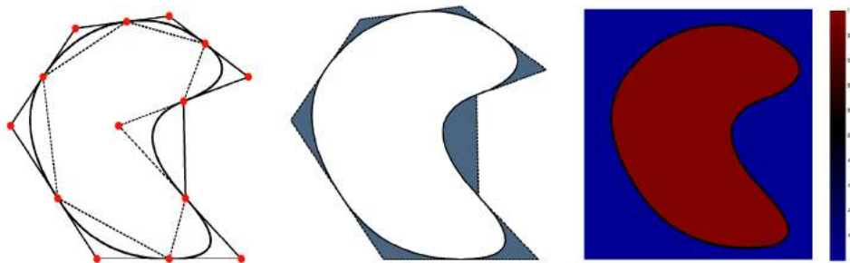
Fig. 8: Signed distance field: (a) Bounding box construction, (b) Shaded regions represent curved Bezier polygons, and (c) Signed field of the closed geometry.
