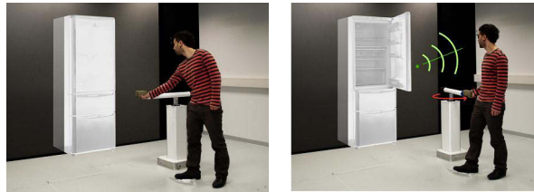
Fig. 3: Phases 2 and 5 of the scenario of use of the mixed prototype: the physical artifact is moved to the right position by the haptic device and the user is able to experience the pre-defined effect asking for some changes.
