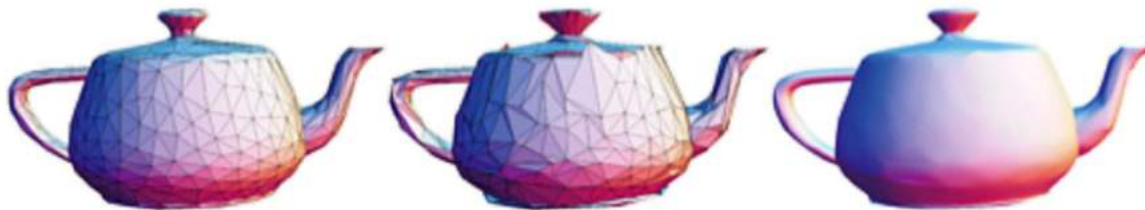
Fig. 2: Example of a failed mesh simplification. Leftmost is the input mesh. Center is the simplified mesh wherein remarkable undulations are seen. Rightmost is the resultant subdivision surface.
