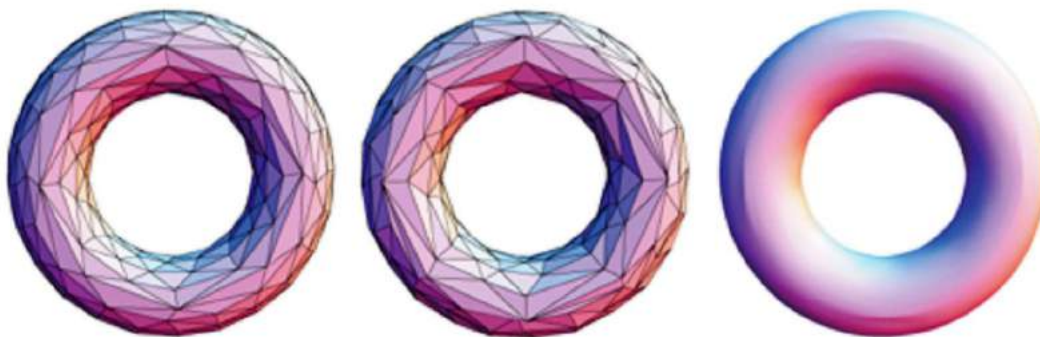
Fig. 7: Input mesh, simplified result by only QEM, and the resultant subdivision surface.
