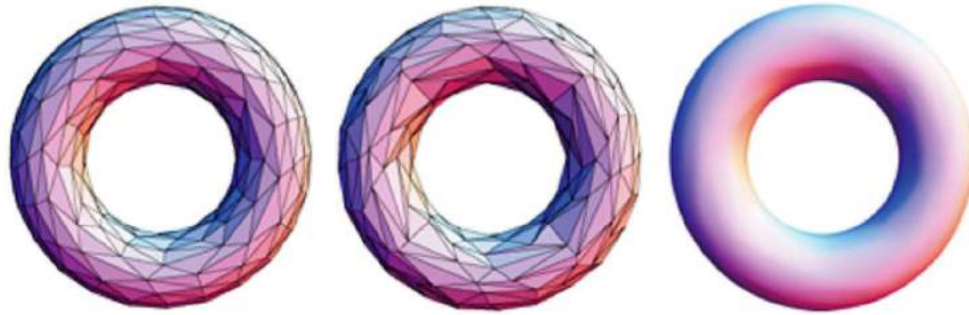
Fig. 8: Input mesh, simplified result by the proposed method, and the resultant subdivision surface.
