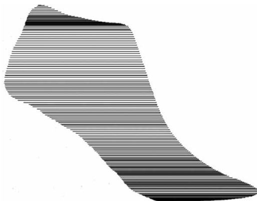
Fig. 17: Adaptive slice of shoe last point cloud using IDS method.
