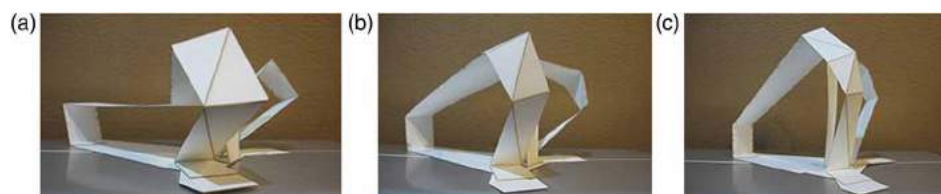
Fig. 13: Models in cardboard, the frog is (a) at rest, (b) raised 21^\circ (c) reach 42^\circ .
