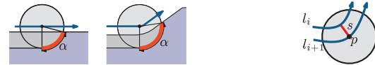
Fig. 2: The engagement angle \alpha at a straight and curved segment of the tool path, and the step-over s . The disk depicts the tool.
