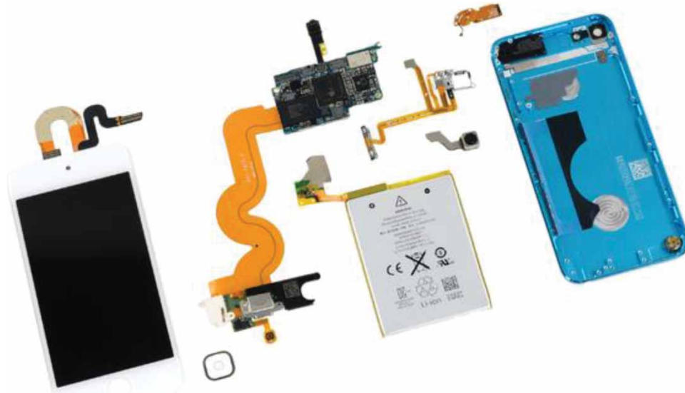
Fig. 1: This photo [6] shows the teardown of an electronic device and several Flexible Printed Circuits (FPCs) (yellow components).
