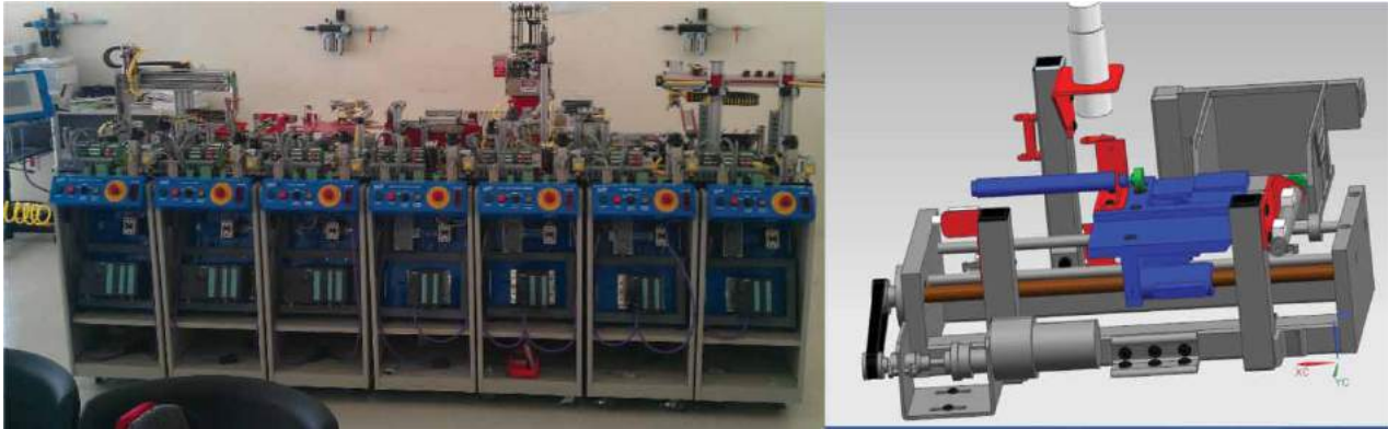
Fig. 1: AMATROL Mechatronics System (left) and Station #2 Gauging drew in NX Software (right).
