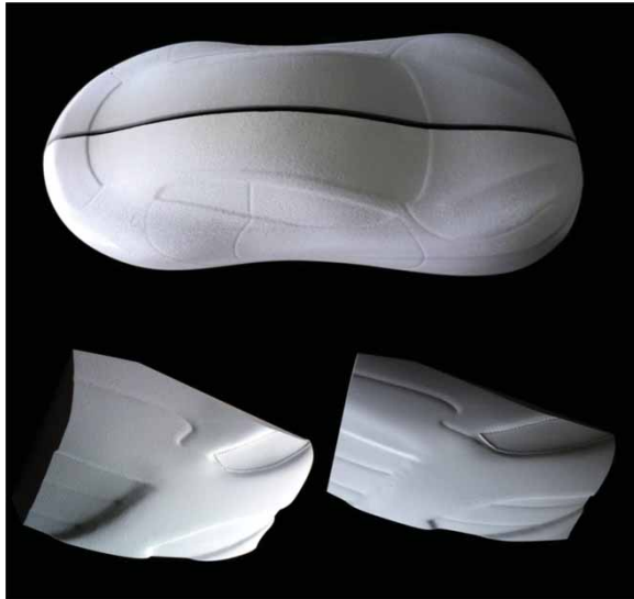
Fig. 9: 1:16 model put against a mirror to see the whole vehicle (top). Two angles of the 1:3 section (bottom).
