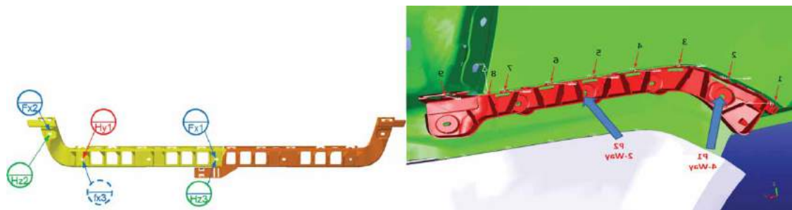
Fig. 12: Optimized locating layout of holders: (a) locating position of Mid-holder (b) locating position of side holder.
