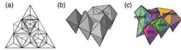
Fig. 14: Modules second level: (a) orthogonal projection, (b) three-dimensional graphical representation and (c) unions, intersections and empty spaces.
