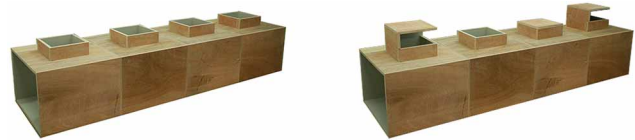
Fig. 1: Physical configurations to generate experimental scenes (left: Even condition; right: Contrast condition).
