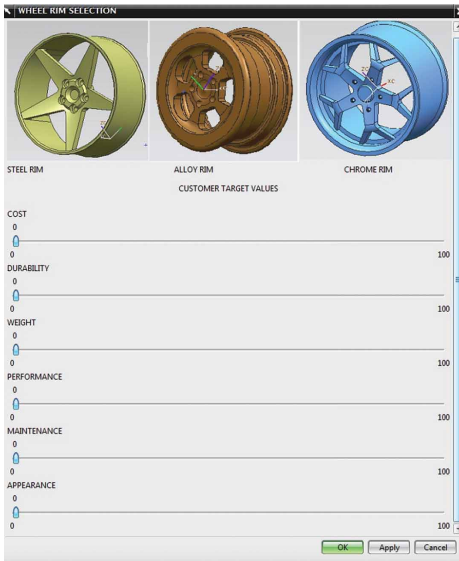
Fig. 4: GUI of KT wheel rim CAD model.
