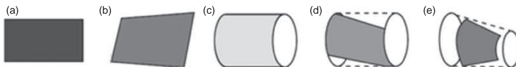
Fig. 4: Atomic shape feature instances: (a) planar rectangular (b) planar polygon (c) cylindrical parallel (d) cylindrical inclined (e) conical.
