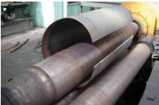
Fig. 3: A rolling machine used to produce cylindrical/conical panels.
