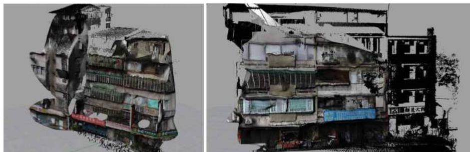
Fig. 9: A merged 3D model of pts file (3D scanner) and obj file (photogrammetry) in Rhino ® to differentiate the foreground (colored polygon model) from the background (points in black color).
