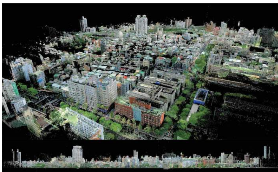
Fig. 1: 3D point cloud model of the district (top) and elevation (bottom).
