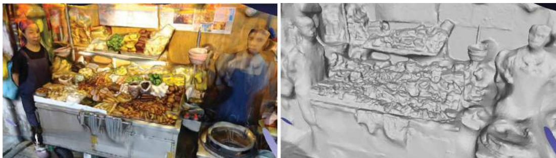
Fig. 8: 3D photogrammetry model of a shop front without image mapped.
