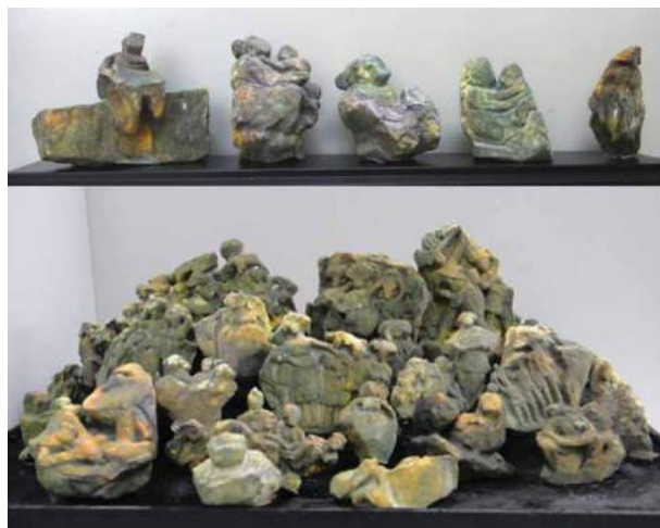
Fig. 10: Illustrating digital data by scaled physical models which are 3D-printed using a RP machine (Microjet®).
