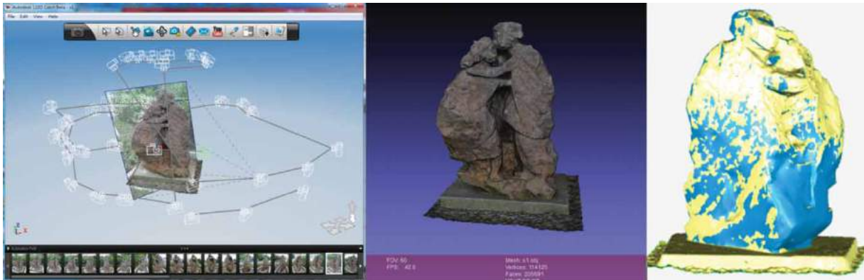
Fig. 14: Photogrammetry creating process (left), 3D model (middle), and the comparison with the model created by 3D scanned data (right).
