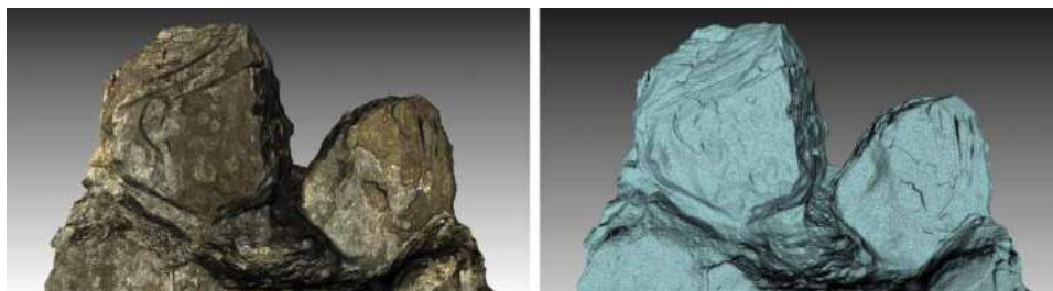
Fig. 4: 3D scanned data with image mapping and in full geometry resolution shown in high density mesh (over 7,000,000 polygons).
