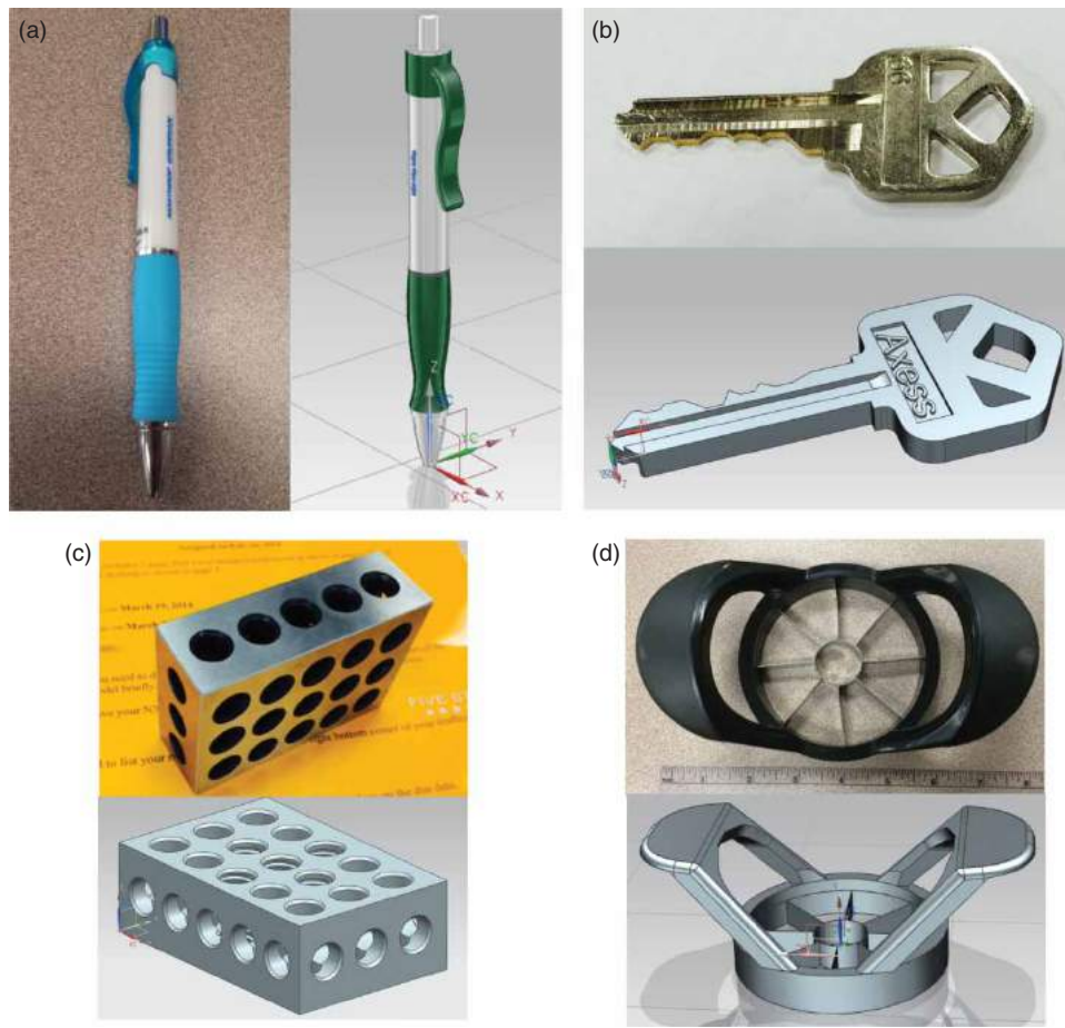
Figure 3. Examples of students' work in four contextual exercises: (a) primitive contextual exercise; (b) remove features contextual exercise; (c) instance contextual exercise; (d) final contextual exercise.
