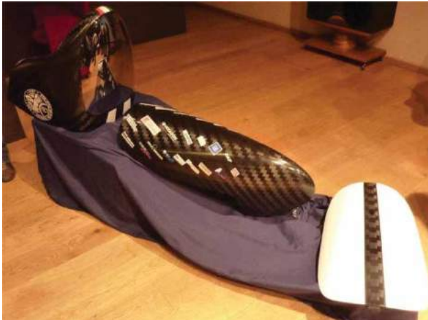
Figure 12. Removable parts of the monocoque in Dynamo Tex.
