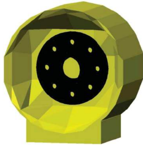
Figure 5. CAD representation of shrinkwrapped wheel and featured hub geometry. Adapter component at the bottom of the wheel is incorporated for vertical load transfer.
