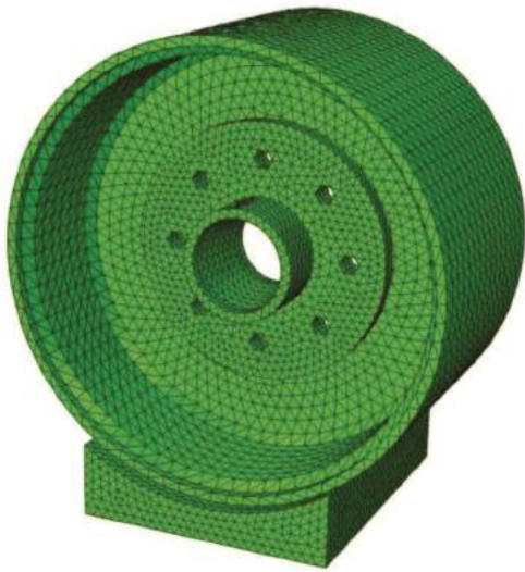
Figure 7. Finite element mesh for full-featured geometry wheel and hub model.
