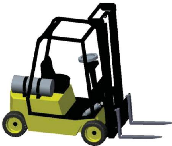
Figure 1. Featured forklift CAD geometry. Forklift is approximately 2.7 m in length, 2.2 m in height and 1.1 m wide with a mass of 3 metric tons [13].
