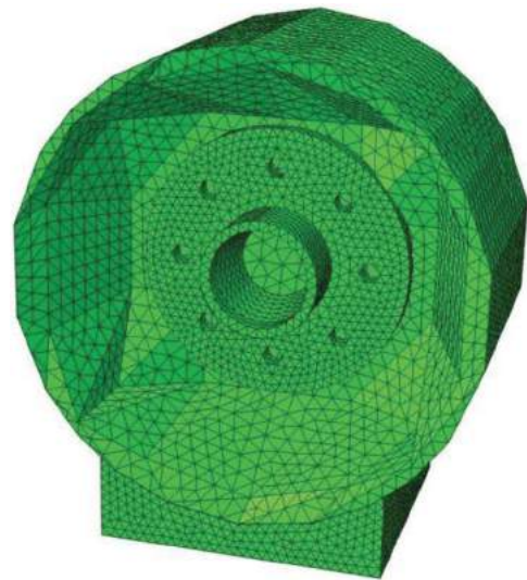
Figure 17. Finite element mesh for shrinkwrap geometry wheel and hub model.
