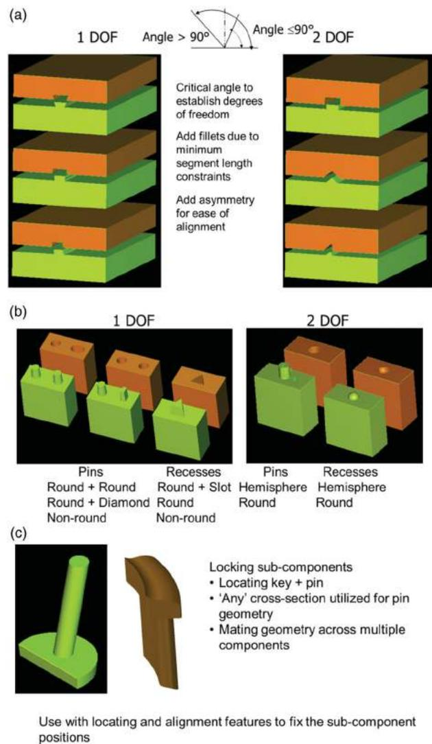
**Figure 12.** (a) Slot geometry with 1 and 2 DOF, (b) boss-hole pair geometry with 1 and 2 DOF, (c) locking pin example (adapted from [40]).
