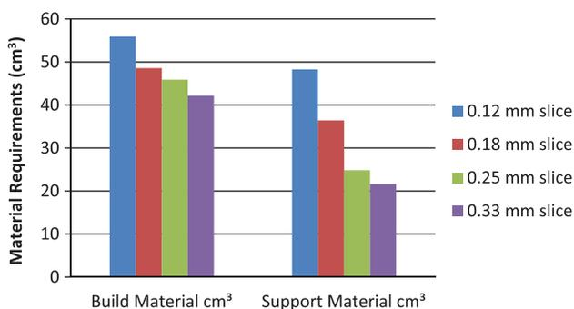
**Figure 6.** Material use variations for a solid fill strategy, with sparse support material, 90° UP build orientation. Note:  $\sim 25\%$  more material is required for the 0.12 mm slice thickness compared to the 0.33 mm slice thickness.
