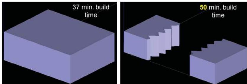
**Figure 11.** The build time for a  $25 \times 25 \times 15$  mm block (0.18 mm slice thickness and solid fill) – one-piece, and the same part with an intricate self-locating interface.
