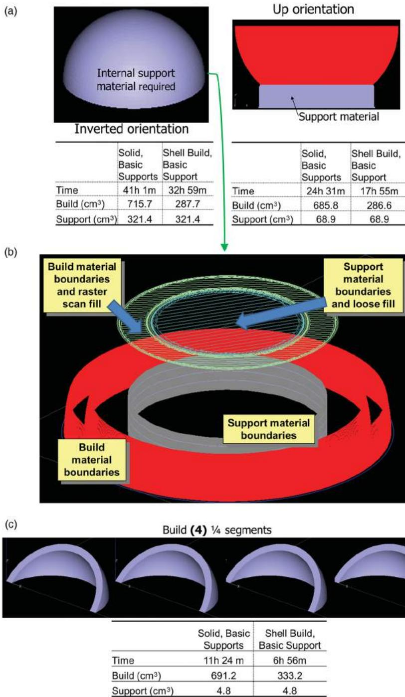
**Figure 7.** The build time and material requirements for 200 mm hemispherical shell with a 12.5 mm wall thickness, built with a 0.18 mm bead height, and a 2:1 ratio of bead width to build height: (a), (b) non-segmented and (c) segmented (all other considerations are constant). Note the minimal amount of support material required for option (c).
