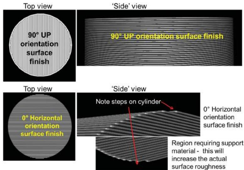
**Figure 4.** The surface finish for the cylindrical body for the two presented build orientations.
