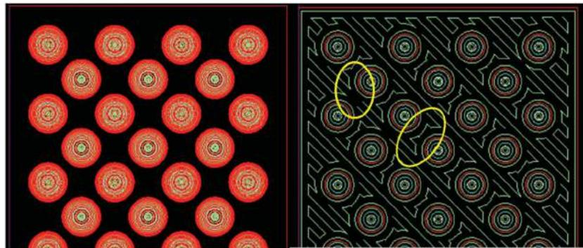
**Figure 14.** Designed voids to reduce the material usage, and voids due to the tool path discontinuities.
