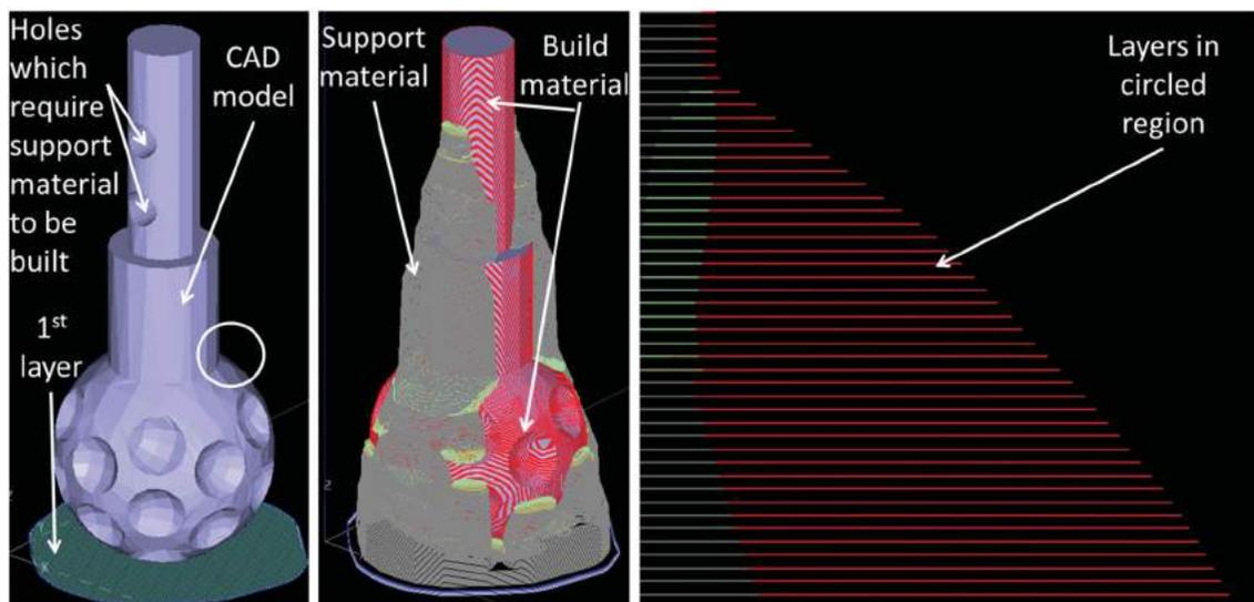
Figure 3. The FDM fabrication for a specialized spherical ball joint.
