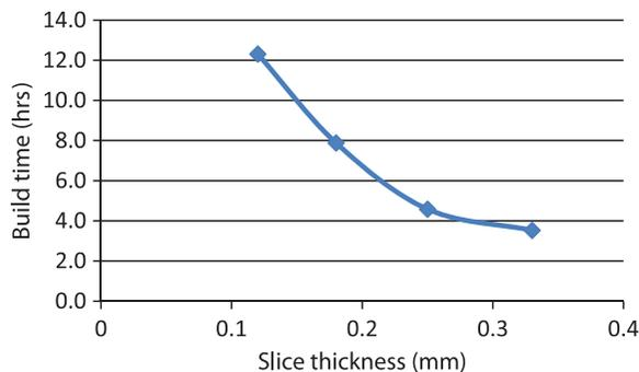
**Figure 5.** Build time variations for a solid fill strategy, with sparse support material, 90° UP build orientation. Note: the trend line has an  $R^2 = 1$  for a polynomial fit, and a trend line fit of an  $R^2 = .99$  for an exponential fit.
