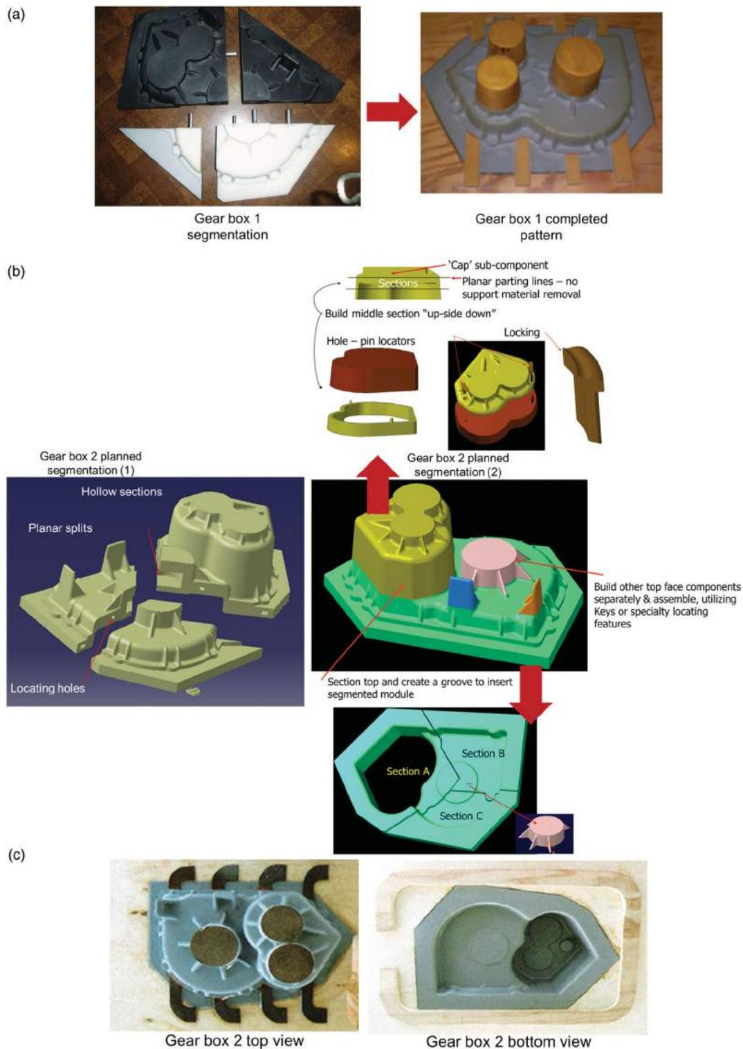
**Figure 16.** (a) Gear box 1 segmentation, (b) Gear box 2 segmentation options, and (c) Gear box 2 final pattern adapted from [40, 41].
