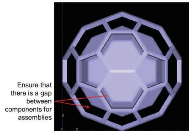
**Figure 9.** A soccer ball within a soccer ball mesh assembly, with a gap.
