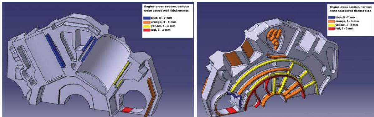
**Figure 17.** Thin wall sections for the V6 block section cope (top) and drag (bottom) – dark blue areas 5–7 mm thick, orange 4–5 mm thick, yellow 3–4 mm thick, red 2–3 mm thick.
