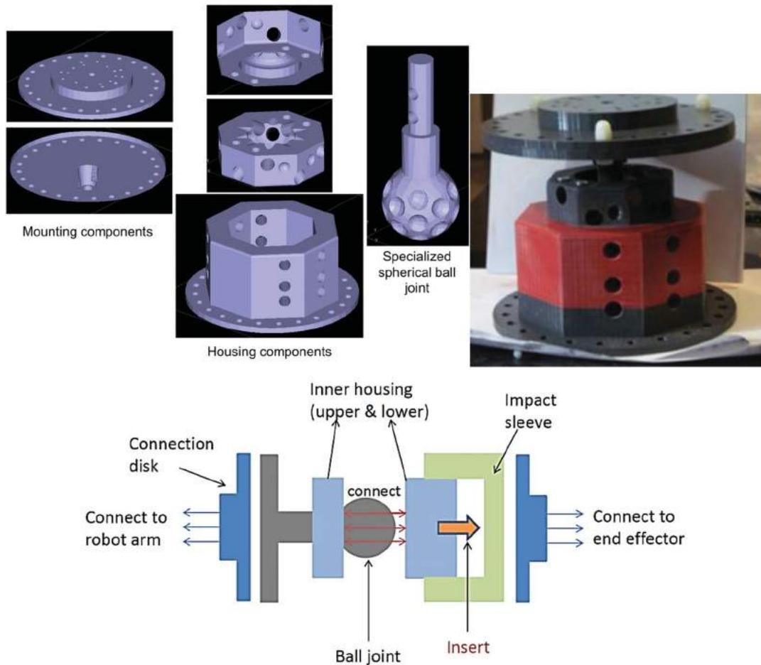
**Figure 19.** Flexible robot end effector coupling components, final FDM model, and the assembly diagram.
