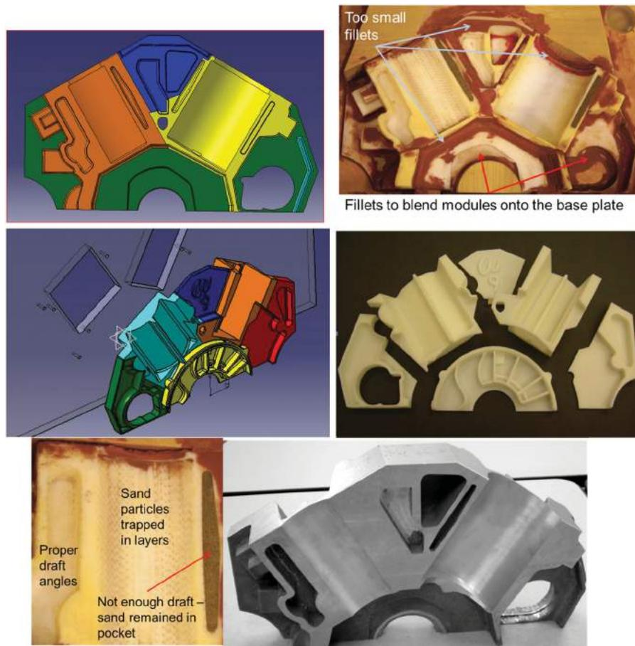
**Figure 18.** V6 block section modules, assembly (cope – top, drag – center), sample module (orange cope module), and final cast part, adapted from [38].
