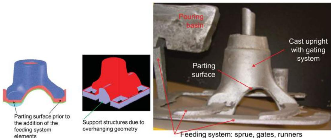
**Figure 15.** The upright casting model, and unfinished casting, adapted from [41].
