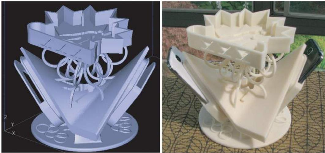
Figure 1. Cell phone charger stand model and built component, illustrating intricate interlocking structures and recessed features.
