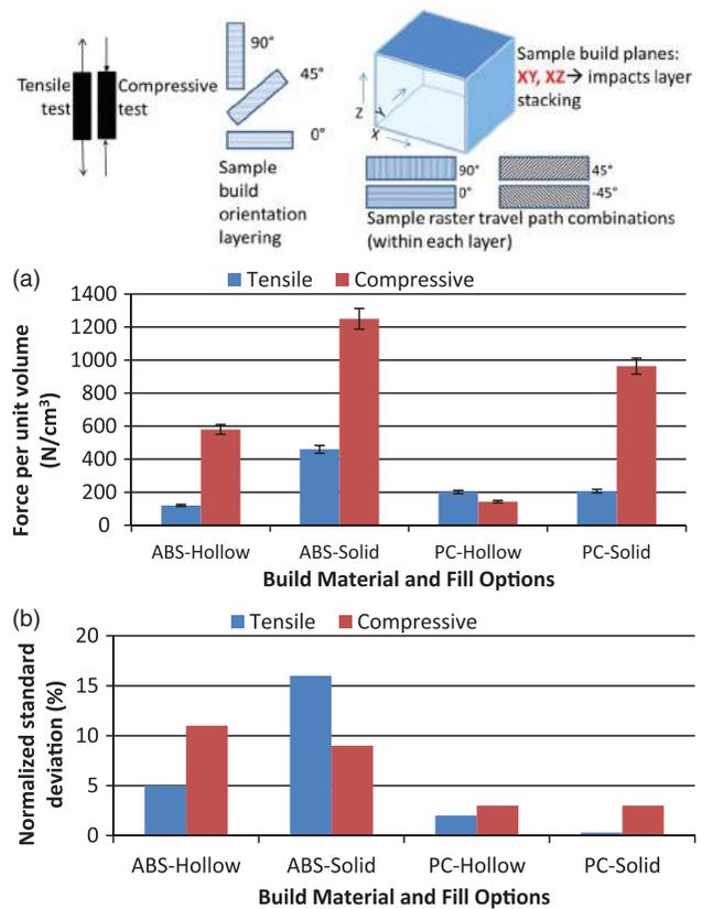
**Figure 13.** (a) The load force per unit volume for solid and hollow test samples for ABS and PC (polycarbonate) materials, and (b) the normalized observed experimental standard deviation.
