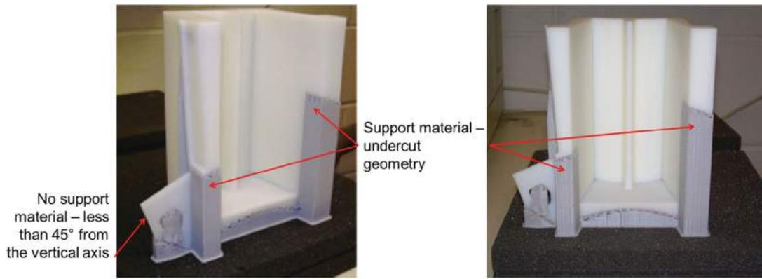
**Figure 10.** The build orientation and the part design influence the amount of support material utilized.
