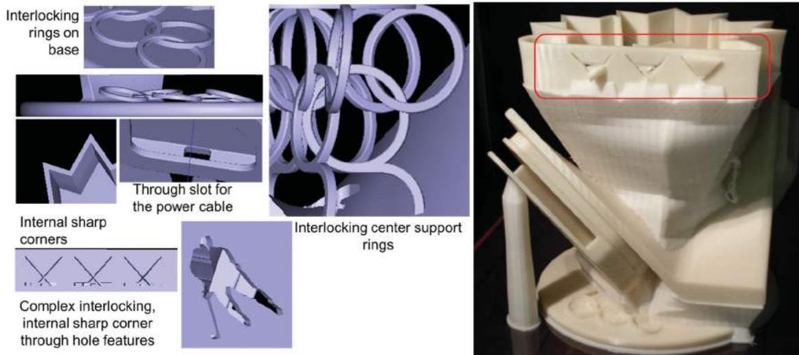
**Figure 20.** Specialty design characteristics for the smart phone holder, and the built model showing the support material, along with problematic build results.
