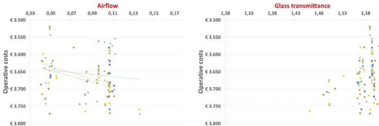
Figure 7. Scatter graphs of optimization variables vs the ranking of the best 100 designs.
