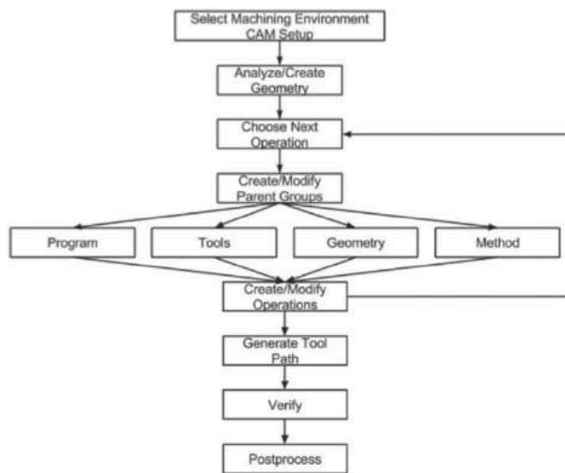
Figure 1. Single user tool path planning loops until every operation has been defined.
