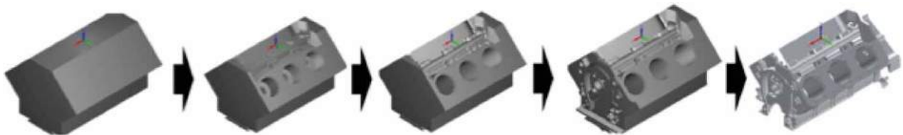
Figure 2. Typical serial progression of operations for an engine block.
