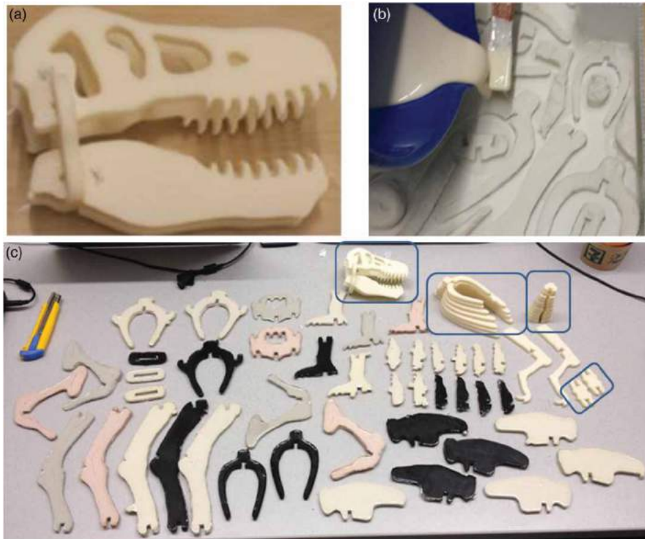
Figure 19. (a) T-Rex head bones built using the FDM process, (b) silicone material being poured into a mold with FDM bone patterns, and (c) molded parts (colored parts were made from resin and a color additive, highlighted head, ribs, and backbones are FDM built parts).
