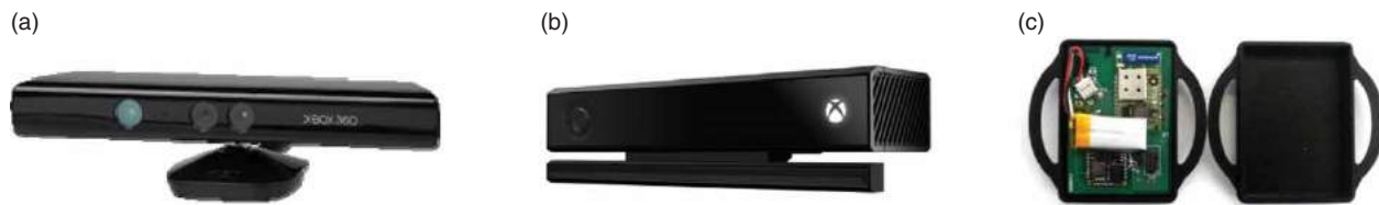
Figure 1. Motion capture devices: a) MS Kinect v1, b) MS Kinect v2, c) wearable inertial sensors.
