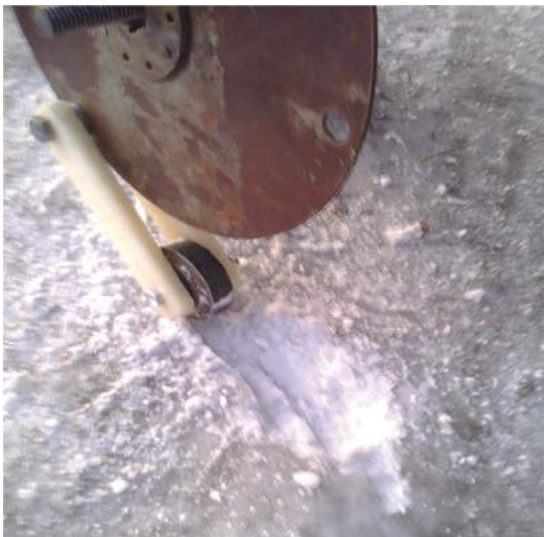
Figure 22. Ice Breaking and Snow Removal Experiment.
