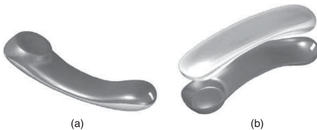
Figure 13. Details of part and product geometry of the modeling example. From left to right: (a) solid model of the exterior, (b) upper and lower housing shell.
