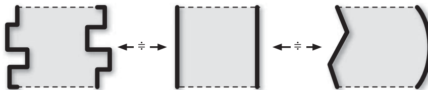
Figure 3. Three different shapes of spaces have the same “SemiOpen” instance of “Openness” property derived from a simplified algorithm, which calculates “EnclosedRate” while ignoring the shape of walls.
