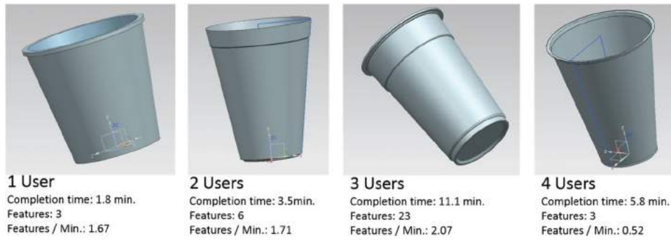
Figure 9. The level of detail included in the model of the cup generally increased with the number of users.
