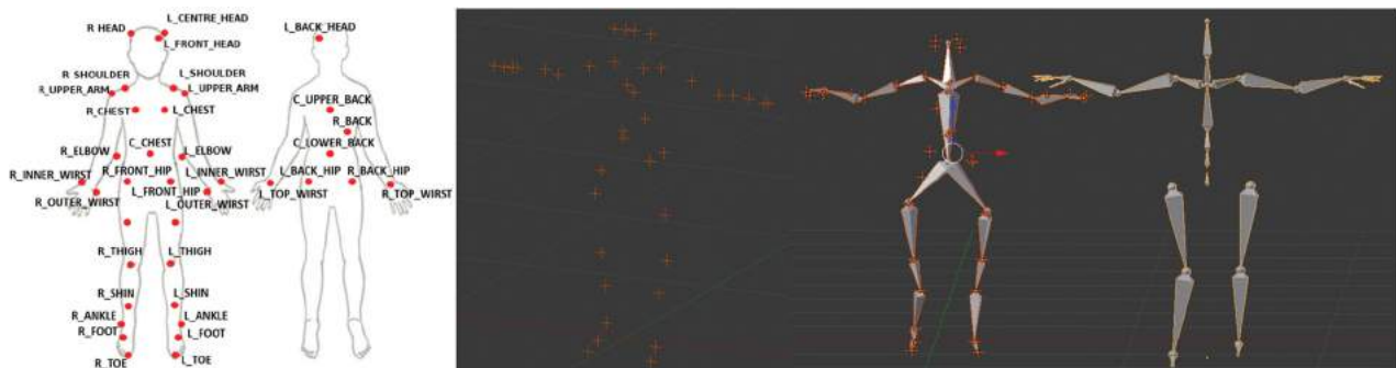
Figure 6. Automatic animation retargeting with MOCAP acquisition by VICON system.
