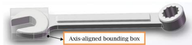
Figure 5. Axis-aligned bounding box of the head of an amphibious wrench model.
