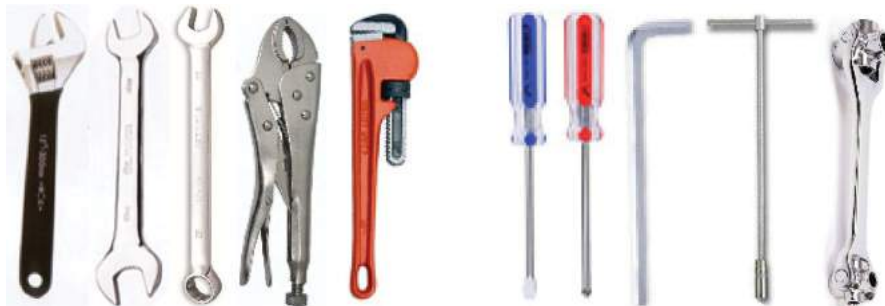
Figure 4. Manual operation tools: (a). Tools rotation not around the fastener axis (b). Tools rotation around the fastener axis.
