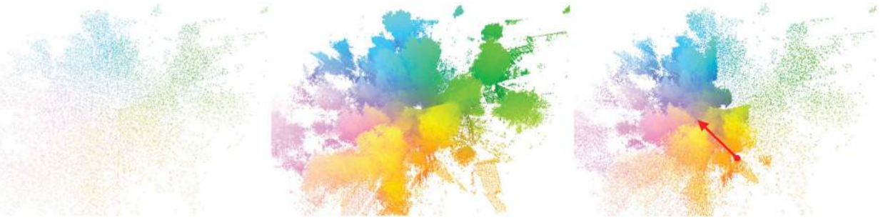
Figure 4. Example of web-based viewing system on Andreas Garten dataset (45M data points). Left shows the data at points from selecting grid levels 0-7 only (48 K data points). The center shows data from grid levels 0-10 (1.1M data points). The right image shows the data points gathered for a view dependent (red arrow) resolution selection (635 K data points).
