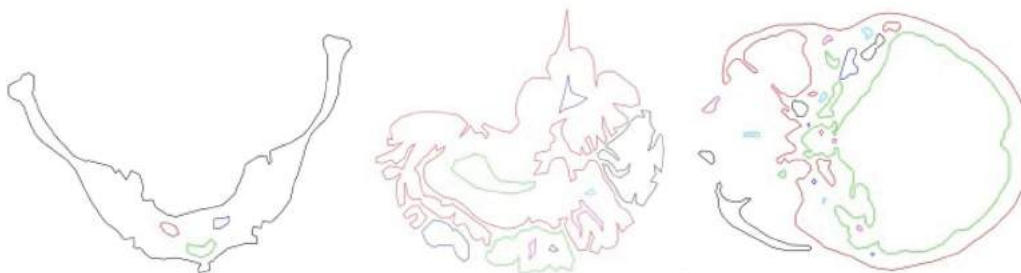
Figure 2. A single slice of a contour dataset typically contains some nested contours and some unnested contours. (a) A pelvis slice. (b) A brain slice. (c) A skull slice.
