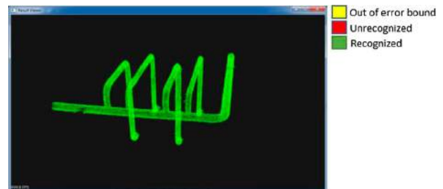
Figure 10. Validating result with the rapid-prototype-based model.
