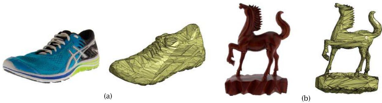
Figure 11. Original images and triangular meshes reconstructed: (a) shoe and (b) horse statue.
