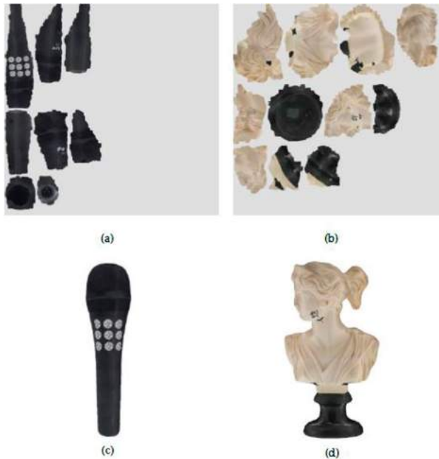
Figure 14. The texture editing and replacing for the “Mic” and “Statue” example, (a) texture edited texture map for the Mic, (b) texture replaced texture map for the Statue, (c) texture edited 3D color model, and (d) texture edited 3D color model.
