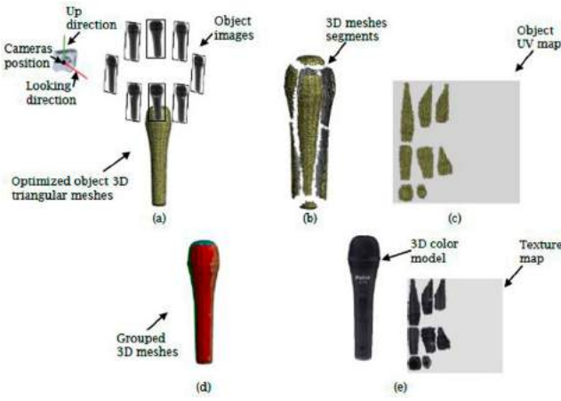
Figure 1. Visualization of the steps of the proposed method, (a) Input object images, camera information, and object meshes, (b) divide 3D meshes into segments for mesh parameterization, (c) unwrap 3D meshes onto the UV domain to yield a UV map, (d) grouping of 3D meshes, and (e) final texture map and 3D color model.
