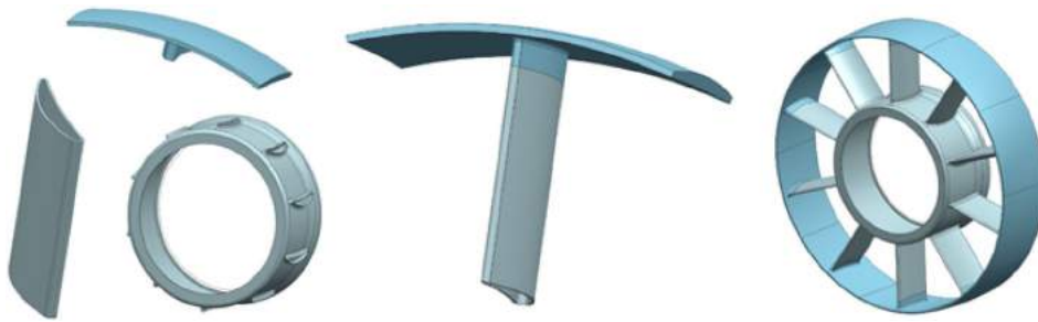
Figure 5. Welding assembly sequence of structural jet engine component.
