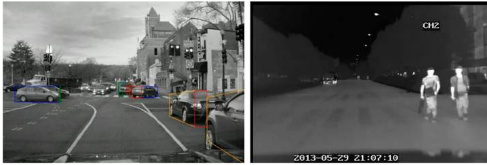
Figure 4. Application of camera systems for object recognition: left daylight camera, right infrared camera, [13], [8].
