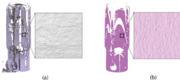
Figure 2. Conversion to wireframe model. a) Point-cloud; b) Wireframe model.
