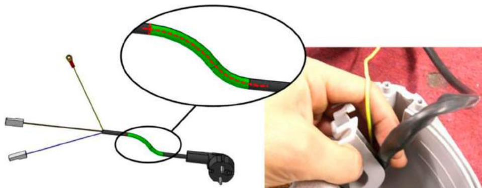
Figure 6. Identification of the critical product feature ( circular section sweep on polylines ) for the cable.
