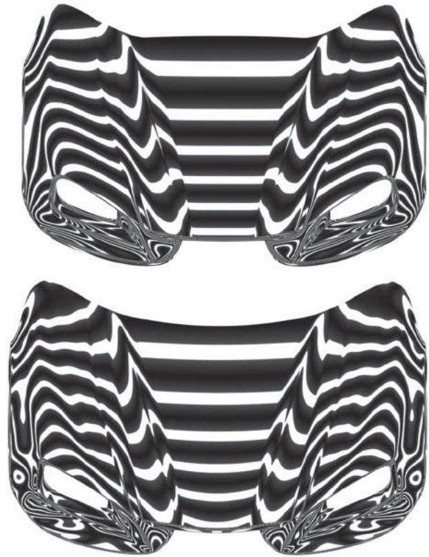
Figure 10. Comparison of highlight diagnoses in ICEM Surf and CATIA.
