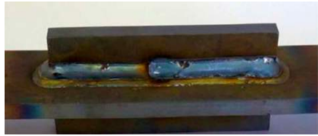
Figure 8. Seam weld (example for a 1d-connection technology) [3].
