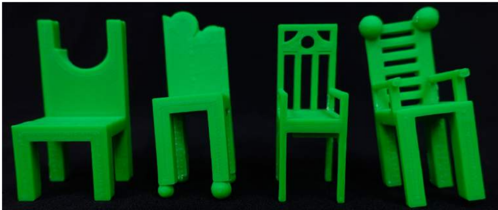
Figure 12. Validation of VR chair models through 3D printed designs.
