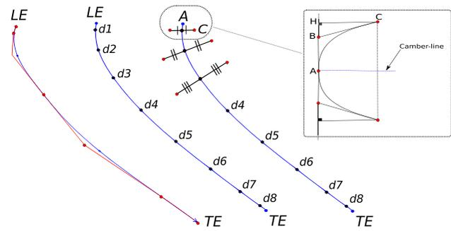
**Figure 4.** Left: Camber-line (blue) with corresponding control polygon (red) and uniform point distribution; Right: Construction of pressure/suction control points; Imposition of curvature (G2 continuity) at the LE
