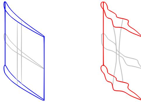
(a) Original stator blade shape (b) Perturbed stator blade shape
