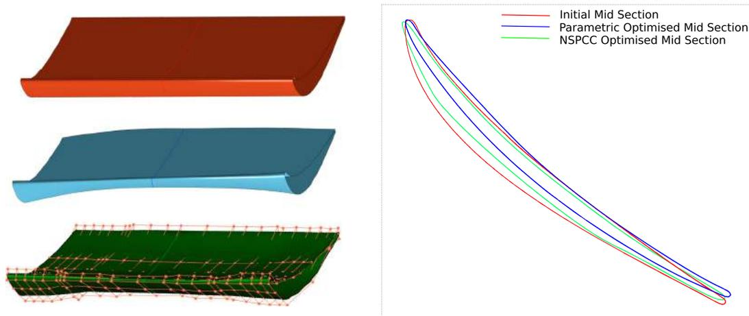
**Figure 11.** Left: Initial TU Stator (red), Optimized Parametric model (blue) and Optimized NURBS (green); Right: Comparison of mid-sections
