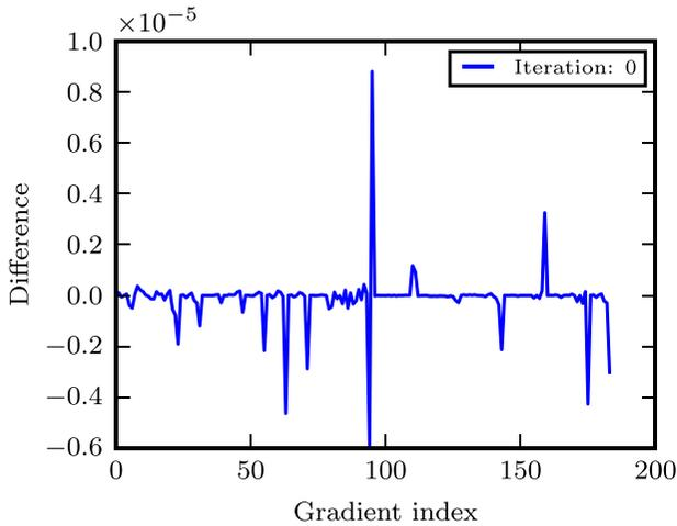
**Figure 3.** Gradient differences between two modes of AD for initial blade optimization iteration
