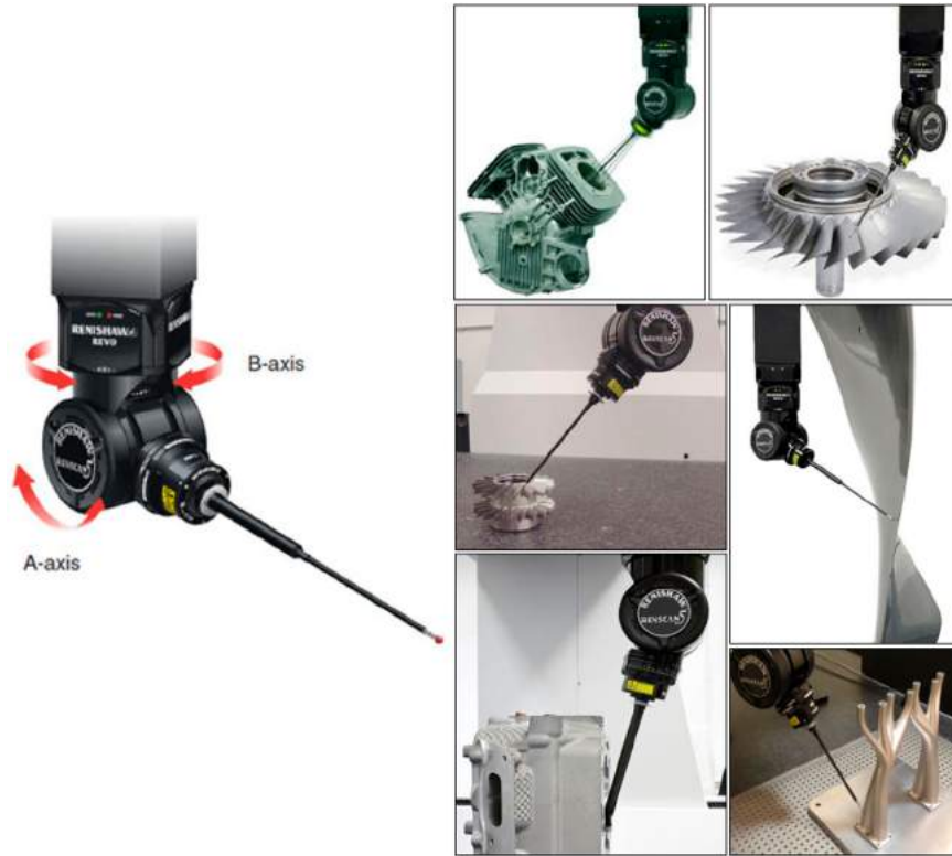
Figure 2. 5-axis CMM (Coordinate Measuring Machine).
