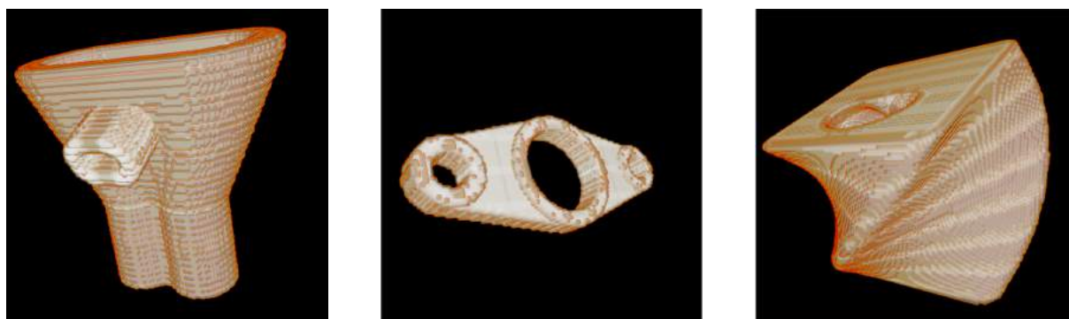
Figure 8: A solid visualization of the implicit boundary representations for three part models. Left to right: multi-plane.stl, widget.stl, and IRAP.stl.
