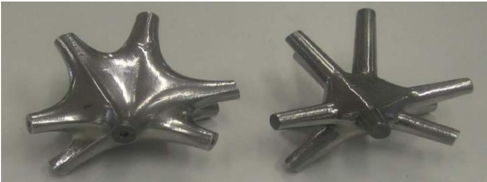
**Figure 26:** Nodes after post-processing (curve parameter node at left, fatness parameter node at right).
