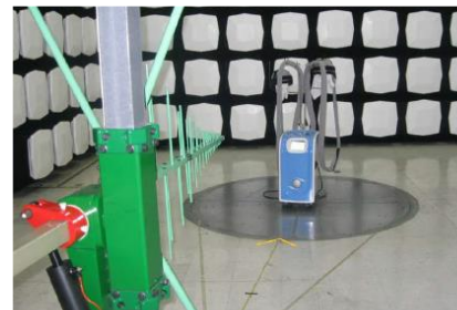
Figure 3: ISO 60601-1 Standard finger test (a), ISO 60601-1-2 Emissions testing (b).
